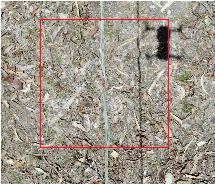
Figure 10 Loosened strands in the test conductor
