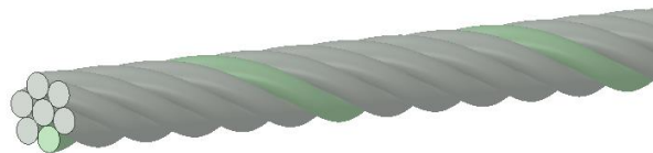
Figure 22 3D CAD model of the 7/.064 copper conductor used for preliminary FEM simulations
