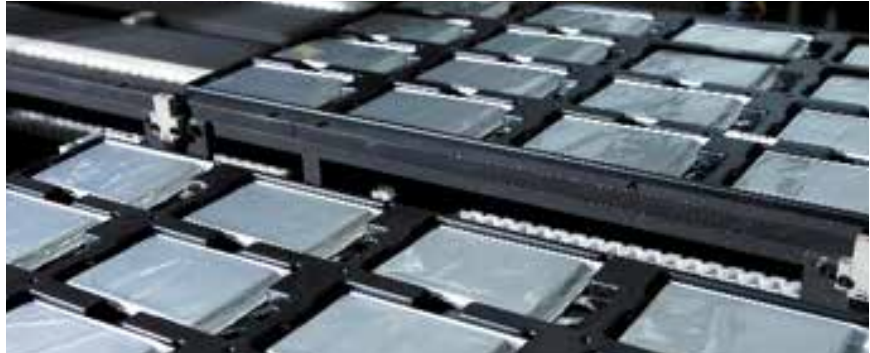
Manufacturing of battery pouches at Kokam's factory in South Korea. There will be approximately 7,900 of these individual battery cells in our 2MW battery.
