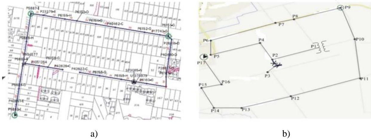
Figure 31 - (a) Urban feeder; (b) rural feeder [8]
